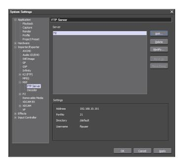
In this screen fill in the details you have set on the T2. With "Connection Test" you can verify that everything works correctly. By failure correct the settings till it passes. Save the configuration by selecting "OK."
